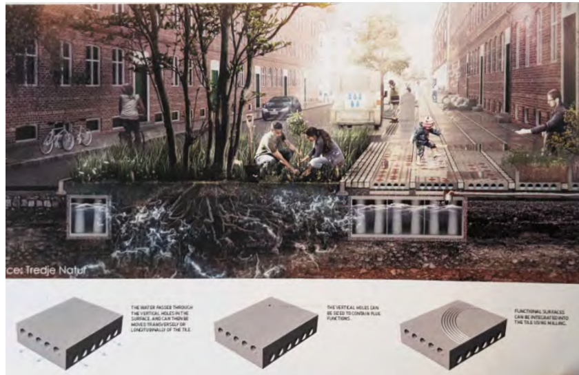
CLIMATE TILE- THE CLIMATE TILE CAPITALIZES ON MAKING NON PERMEABLE PAVEMENT PERMEABLE. WATER CAN BE HELD TO REDUCE DOWNSTREAM FLOODING AND BE FILTERED THROUGH THE TILE AND BACK INTO THE URBAN WATER SYSTEM
