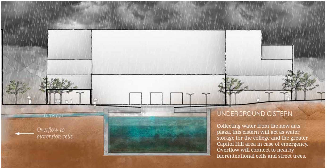
Underground Cistern Section (nts)
