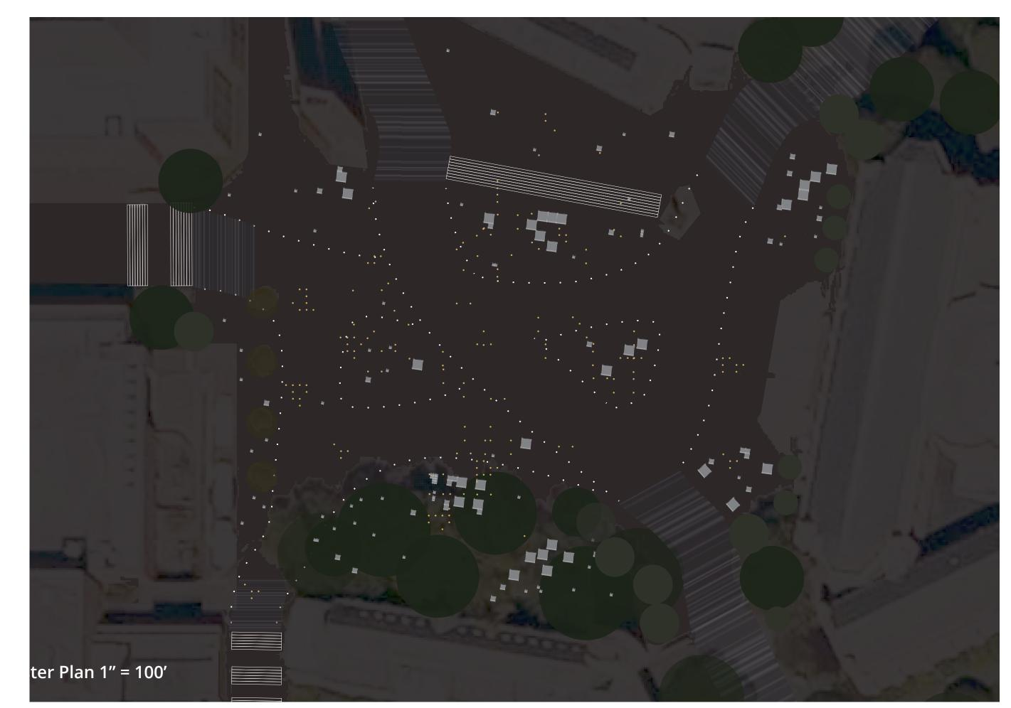
The illuminated pavement will harvest energy from pedestrian footsteps during the day, and reveal the "desire paths" they create through the square at night. These paths will serve as wayfinding for ADA accessible routes through campus. During the evening and night the paving will light up underneath the footsteps of each visitor, allowing them to light their own way. The playfulness of pressure activated pavement invites people to come, enjoy, and creatively engage with light in the square.
