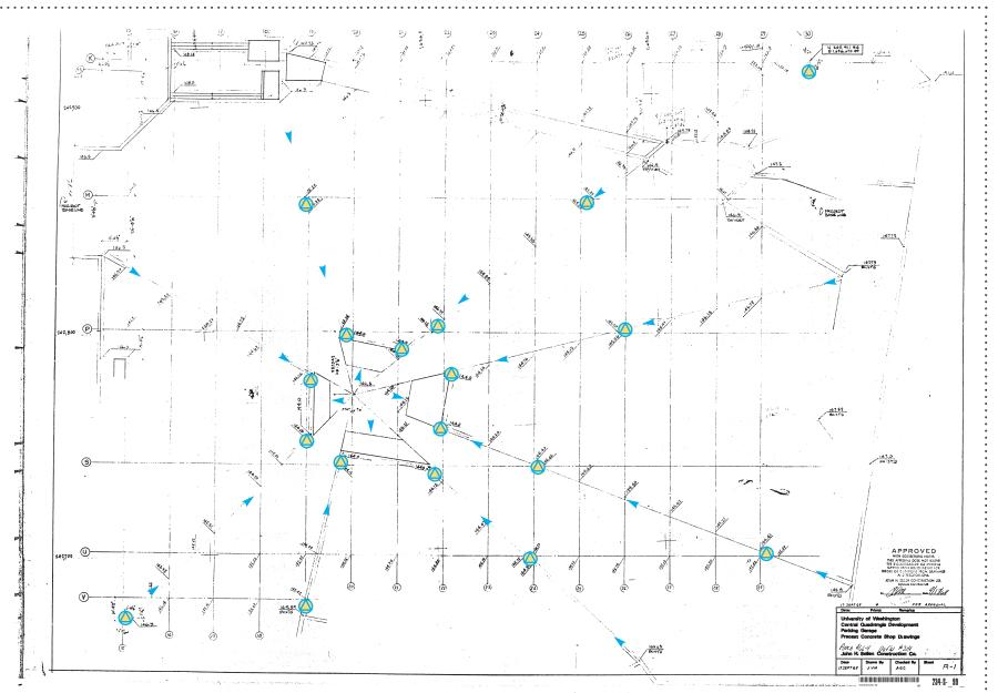
**DRAINAGE OVER THE PARKING GARAGE** - The roof over the parking garage is cast-in-place concrete and has already been sloped toward the center of the plaza. The very center is slightly mounded so that water moves towards drains near each of the four benches. Other drains are located in the cement lines radiating out from the center. These drains would be difficult to site elsewhere.
